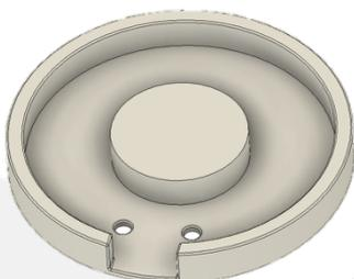
Design engineers often add break edges onto parts to remove sharp edges, sometimes this is warranted to ensure insulation breakdown doesn't occur over time or on high voltage applications it can remove arcing.
