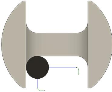
To achieve less than 0.5mm would require a separate setup routine which sets the corner parallel with the Z axis, even with this separate setup, the sharp corner rule still applies which would leave a rad of 0.4mm MAX or 0.2mm Max if the finishing technique was used.
