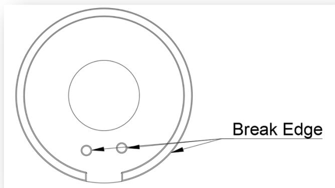
When the parts are pressed, it is useful to have a break edge to allow for a homogenous pressing density and to allow the core to be easily removed from the tool.
