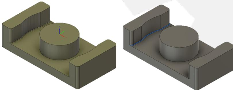
The internal corners of the core cannot be 90 degrees within the Z-axis plane, corners must have an internal radius for both machining and pressing. In pressing this is related to how the core is pressed and ensuring a consistent pressing density throughout the core. In Machining, this is related to how the cutting tools are manufactured, the tools need to provide sufficient surface area to hold the abrasive cutting compound, this means that tools cannot be made with a 90-degree corner.
