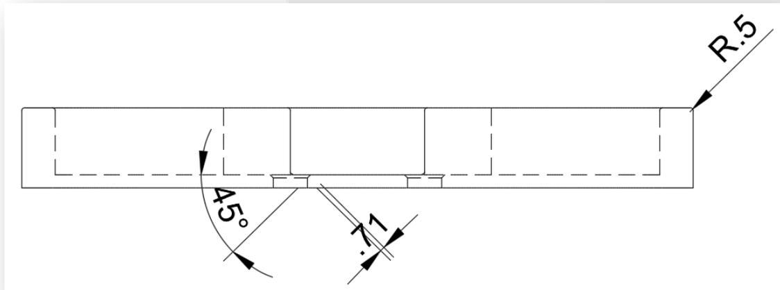
Any other edge that is designed to incorporate a break, that doesn't have a positive impact on electrical/magnetic performance, should be labelled as a break edge, in this scenario the team would apply a small chamfer to these edges.
