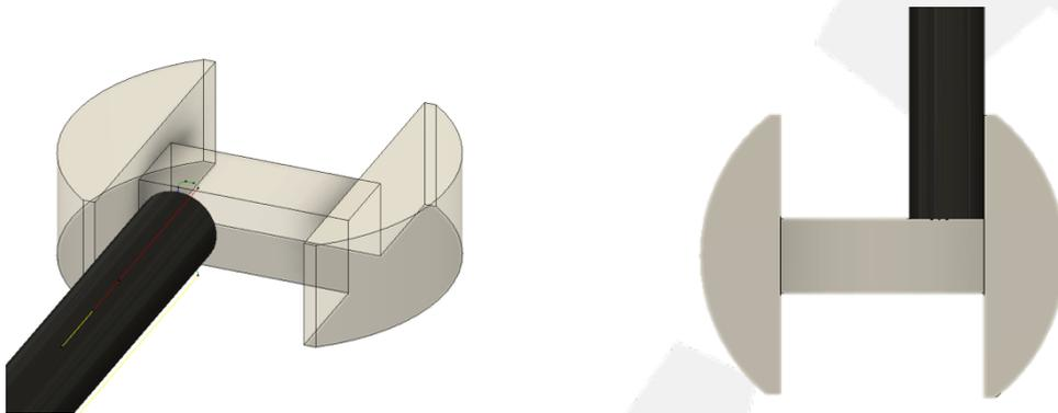
This limitation is only relevant to machining ferrite, sharp corners can be pressed in the X and Y Axis with a minimal radius.
